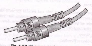
Fig. 4.8.2 ST connector for fiber cable
