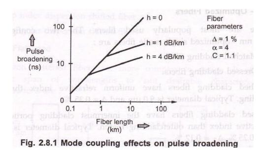
• Significant mode coupling occurs of connectors, splices and with other passive components of an optical link.
