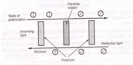
Fig. 7.4.1 Isolator works only for a particular state of polarization
