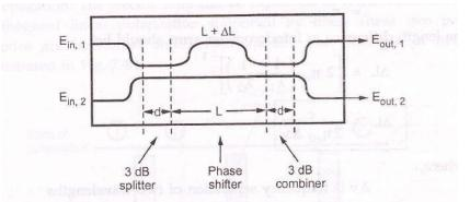
Flg. 7.3.1 Layout of 2×2 passive Mach-Zehnder Interferometer
