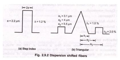
• The addition of wavelength and material dispersion can shift the zero dispersion point of longer wavelength. Two configurations of dispersion shifted fibers are :
