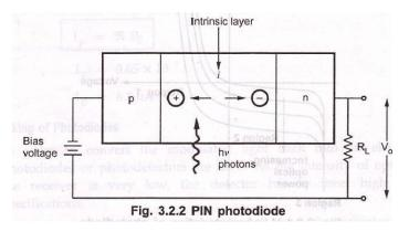
• Sufficient reverse voltage is applied so as to keep intrinsic region free from carries, so its resistance is high, most of diode voltage appears across it, and the electrical forces are strong within it. The incident photons give up their energy and excite an electron from valance to conduction band. Thus a free electron hole pair is generated, these are called
