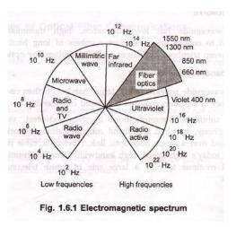
• Fiber optics uses visible and infrared light. Infrared light covers a fairly wide range of wavelengths and is generally used for all fiber optic communications. Visible light is normally used for very short range transmission using a plastic fiber.
