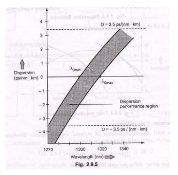
• Maximum dispersion specified as 3.5 ps/(nm . km) marked as dotted line in Fig. 2.9.5.
