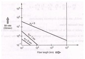
Fig. 2.6.5 Dependence of bit rate on fiber length
