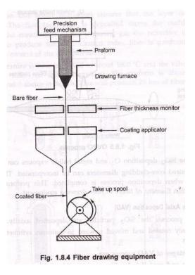
• The fiber thickness monitoring decides the speed of take up spool. The fiber is then coated with elastic material to protect it from dust and water vapour.
