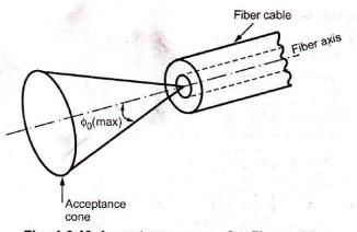
Fig. 1.6.10 Acceptance cone of a fiber cable
