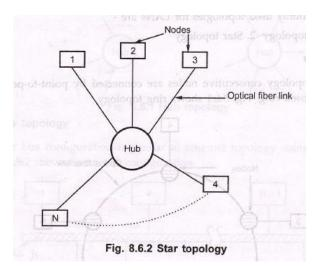
• LANs in star topology can further be classified into active star networks and passive star networks depending on whether the central hub is active or passive device.
