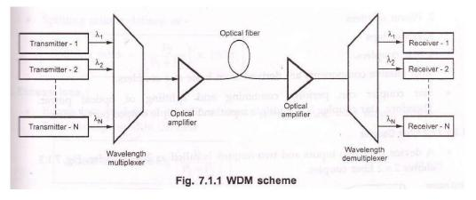
• To prevent spurious signals to enter into receiving channel, the demultiplexer must have narrow spectral operation with sharp wavelength cut-offs. The acceptable limit of crosstalk is – 30 dB.
