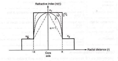
Fig. 1.6.15 Possible fiber refractive index profiles for different values of  $\boldsymbol{\alpha}$
