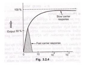
• The detector behaves as a simple low pass RC filter having passband of
