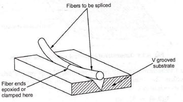
Fig. 4.2.2 V groove optical fiber splicing technique
