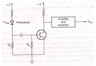
Fig. 5.1.5 High input impedance preamplifier using FET
