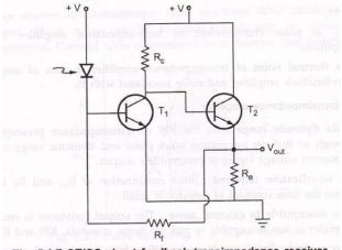
Fig. 5.1.7 CE/CC shunt feedback transimpedance receiver
