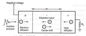
Fig. 3.2.3 Reverse biased PIN diode
