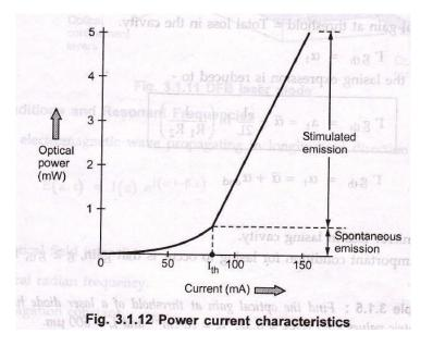
Fig. 3.1.12 Power current characteristics
