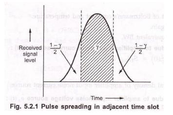
• Intersymbol interference (ISI) also contributes to error which is causing from pulse spreading. Because of pulse spreading energy of a pulse spreads into neighbouring time slots, results in an interfering signal. Fig. 5.2.1 shows ISI.
