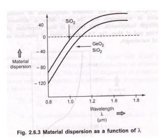
• The unit of dispersion is : ps/nm . km. The amount of material dispersion depends upon the chemical composition of glass.
