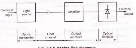
Fig. 6.1.1 Analog link elements
