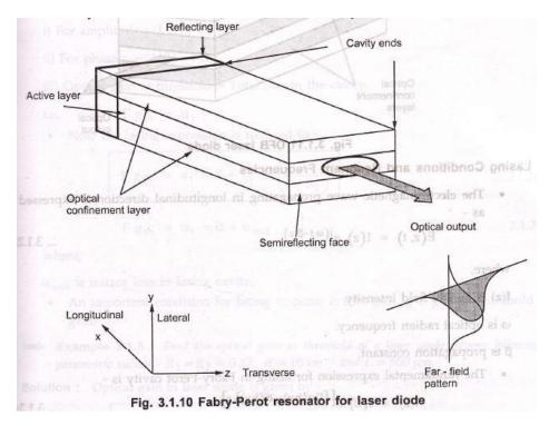
Light propagating along the axis of the interferometer is reflected by the mirrors back to the amplifying medium providing optical gain. The dimensions of cavity are 25-500  $\mu$ m longitudinal 5-15  $\mu$ m lateral and 0.1-0.2  $\mu$ m transverse. Fig. 3.1.10 shows Fabry-Perot resonator cavity for a laser diode.
