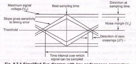
Fig. 8.7.4 Simplified Eye-diagram with key performance parameters
