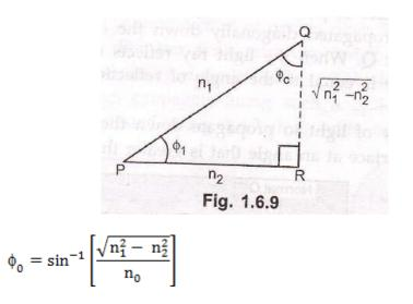
The maximum value of external incidence angle for which light will propagate in the fiber.
