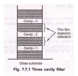
• For configuring a multiplexer and demultiplexer, a number of such filters can be cascaded. Each filter passes a different wavelength and reflects other. While using as demultiplexer, the filter in cascade passes one wavelength and reflects all others onto second filter. The second filter passes another wavelength and reflects remaining wavelengths.
