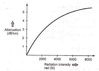
Fig. 2.2.1 lonizing radiation intensity Vs fiber attenuation
