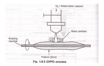
• During the SiO<sub>2</sub> deposition O<sub>2</sub> and metal halide vapours can be controlled so the desired core-cladding diameters can be incorporated. The mandrel is removed when deposition process is completed, This preform is used for drawing thin filament of fibers in fiber drawing equipment.
