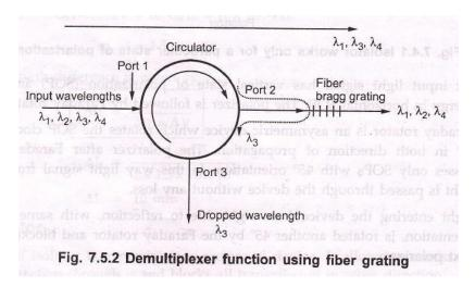
• The circulator takes four wavelengths  $\lambda 1$ ,  $\lambda 2$ ,  $\lambda 3$  and  $\lambda 4$  from input port-1 tunable filter operates on similar principle as passive devices. It operates over a range of frequencies and can be tuned at only one optical frequency to pass through it. Fig. 7.6.1 illustrates concept of tunable filter.
