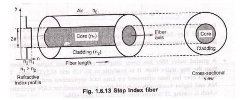
• The propagation of light wave within the core of step index fiber takes the path of meridional ray i.e. ray follows a zig-zag path of straight line segments.
