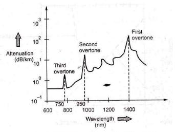
Fig. 2.2.2 Absorption spectra for OH group
