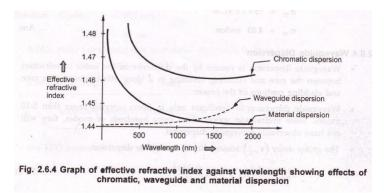
• Material dispersion and waveguide dispersion effects vary in vary in opposite senses as the wavelength increased, but at an optimum wavelength around 1300 nm, two effects almost cancel each other and chromatic dispersion is at minimum. Attenuation is therefore also at minimum and makes 1300 nm a highly attractive operating wavelength.
