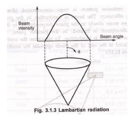
• The power is reduced to 50% of its peak when  $\theta = 60^{\circ}$ , therefore the total half-power beamwidth is 120°. The radiation pattern decides the coupling efficiency of LED.
