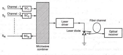
Fig. 6.1.5 Sub-carrier multiplexing
