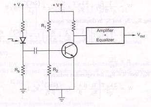
Fig. 5.1.6 High input impedance preamplifier using BJT
