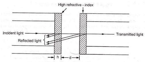
Fig. 4.8.6 Reflections from fiber end faces
