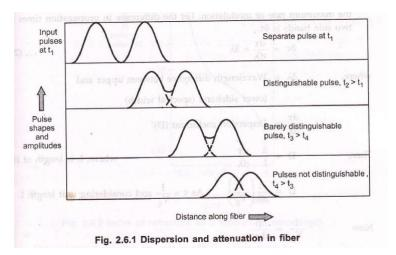
• Fig. 2.6.1 shows, after travelling some distance, pulse starts broadening and overlap with the neighbouring pulses. At certain distance the pulses are not even distinguishable and error will occur at receiver. Therefore the information capacity is specified by bandwidth-distance product (MHz . km). For step index bandwidth distance product is 20 MHz . km and for graded index it is 2.5 MHz . km.
