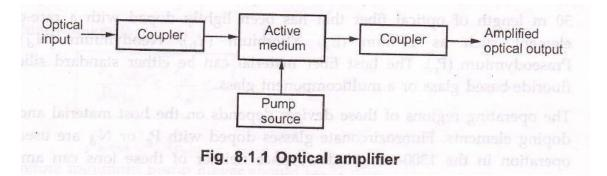
medium. The electrons shifts to the higher energy level producing population inversion. Photons of incoming signal triggers these excited electrons to lower level through a stimulated emission process, producing amplified optical signal.
