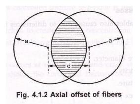
• The optical power coupled is proportional to common area of two fiber cores. The common area is given by expression –
